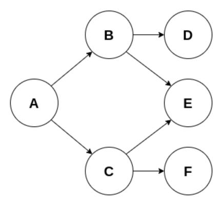
In the example above, node A depends on nodes B and C; node B depends on nodes D and E; node C depends on nodes E and F. Nodes D, E and F are the independent nodes and take the initial positions. A dependency graph may have multiple topological orders. Some valid topological orders for the graph above are:
