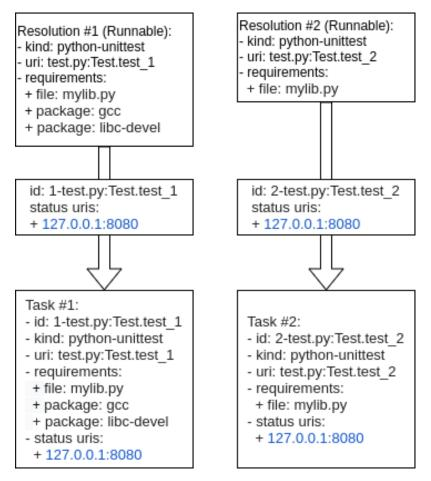
In the end, a job will contain a test\_suite with "Task #1" and "Task #2". It means that the execution of both tasks was requested by the Job owner.
