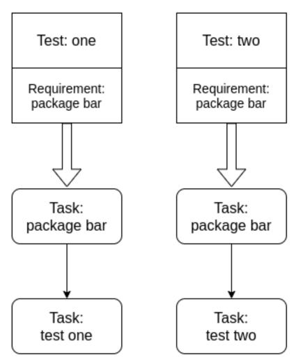
The straightforward solution to this problem is to identify the same requirement for multiple tests in the same environment and create one single task for this requirement. This solution is limited to tests and their requirements. Another idea, and the proposal of this blueprint, is to expand the Requirements Resolver to a Dependency Graph.
